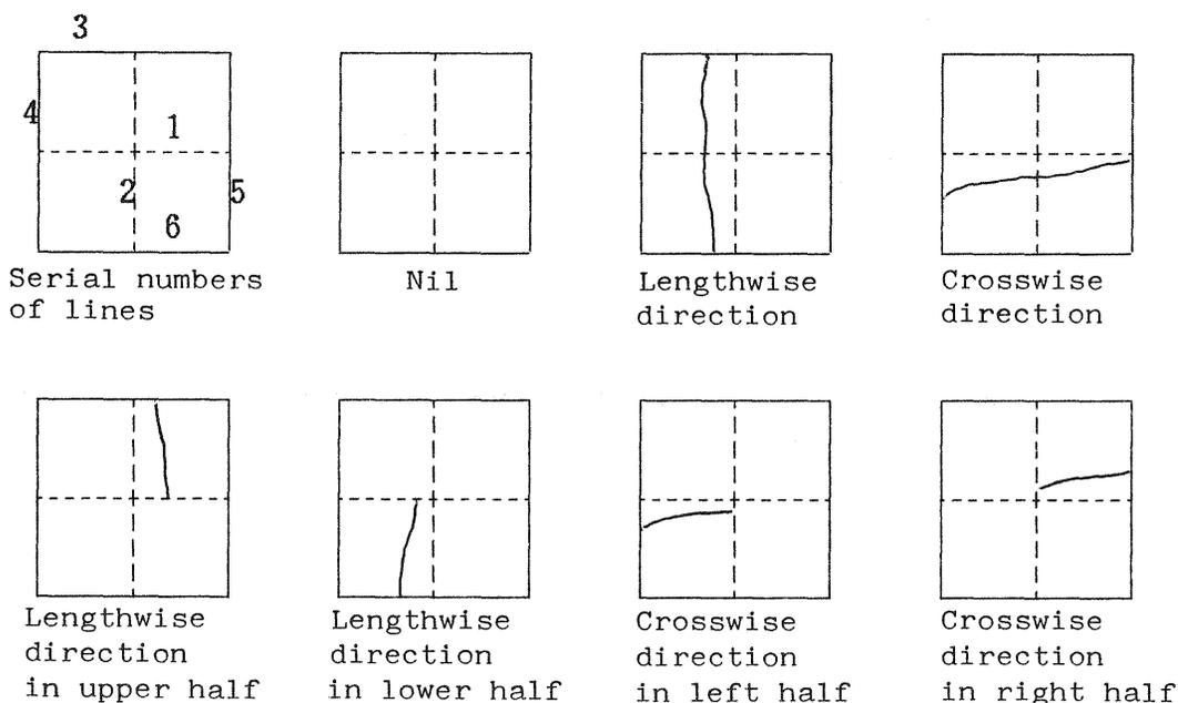
If the points with possibility of having cracks have not been detected on lines 1 and 2 or continuity has not been recognized, then there are no cracks, and you should thus, move to the next small square.
