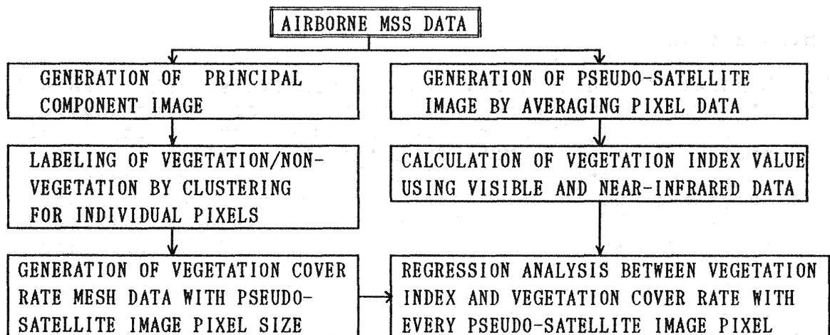
Fig.1 Flow chart of simulation experiment for the estimation of vegetation cover rate within one pixel size of satellite images using vegetation index as a spectral feature.
