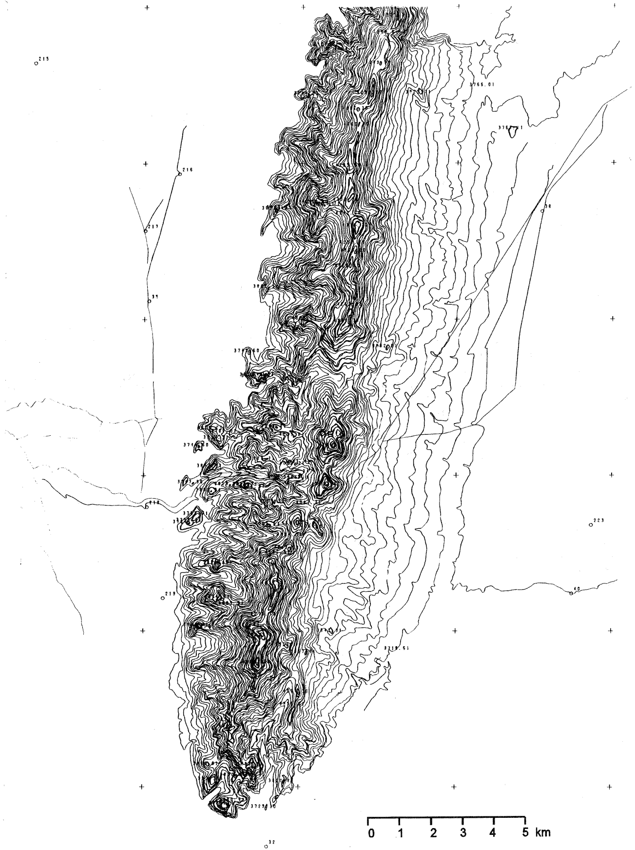
Figure 7. Experimental elevation contour plot with 20m contour interval (Bolivia scene)
