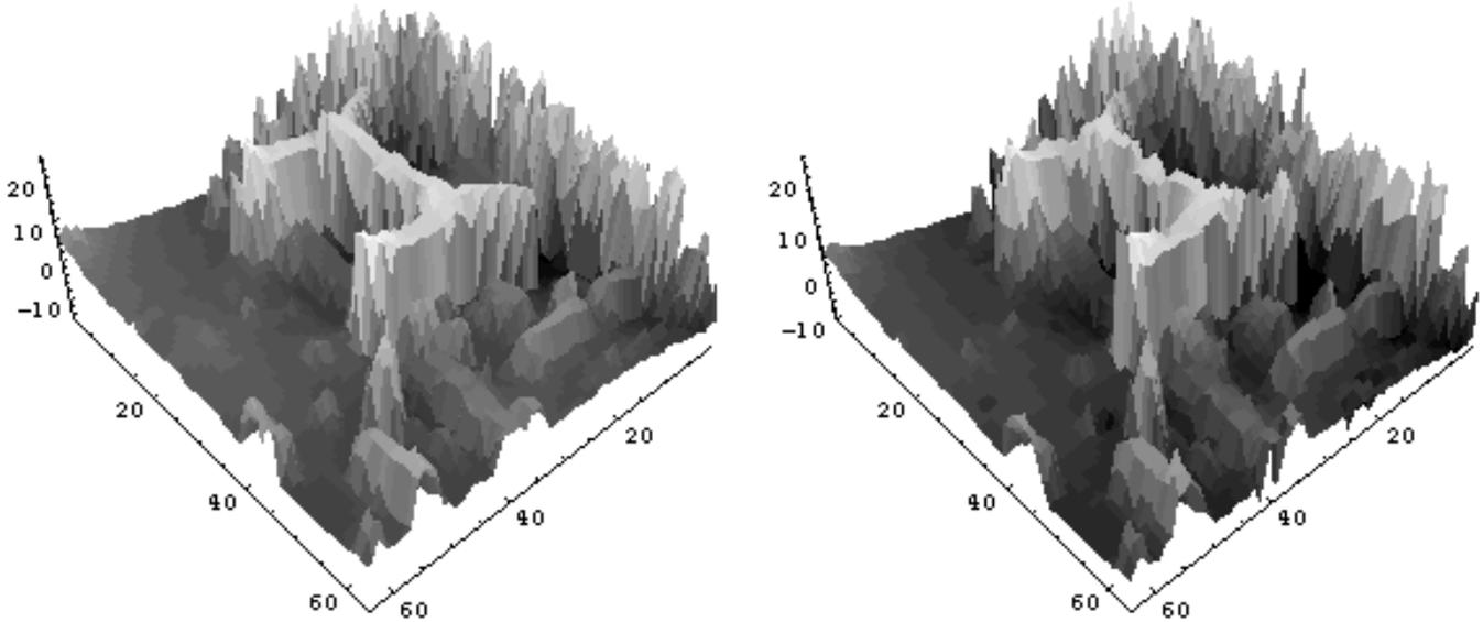
Figure 6: the original LIDAR of a large structure in the Presidio area (*left*) and its reconstructed planar patch approximation (*right*)
