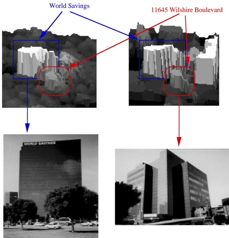
Figure 1: The original (*top left*) and extracted shapes (*top right*) of two buildings in S. Monica, Los Angeles. The starting data was a 2.5 m posting TOPSAR DTM.
