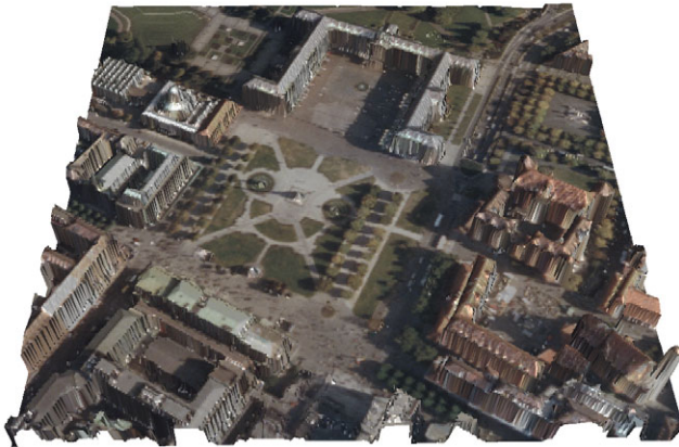
Figure 1 DSM from laser scanning with aerial image overlaid
