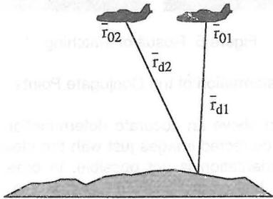
Figure 7: Reconstruction of an object point
