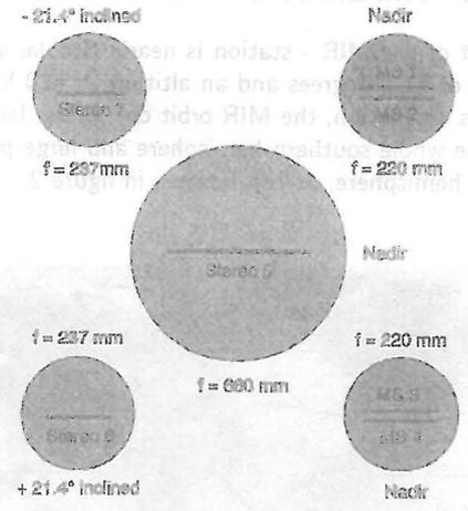
Figure 6: Optical parameters of the five objectives
