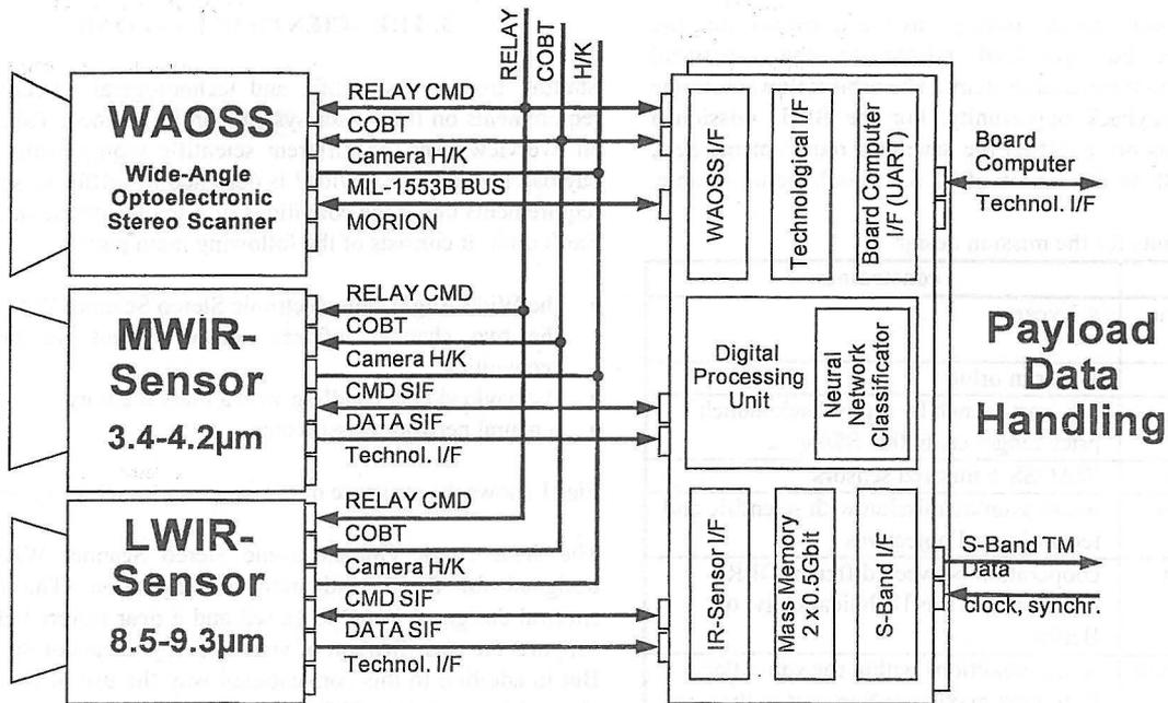
Fig. 1: Scientific payload of BIRD
