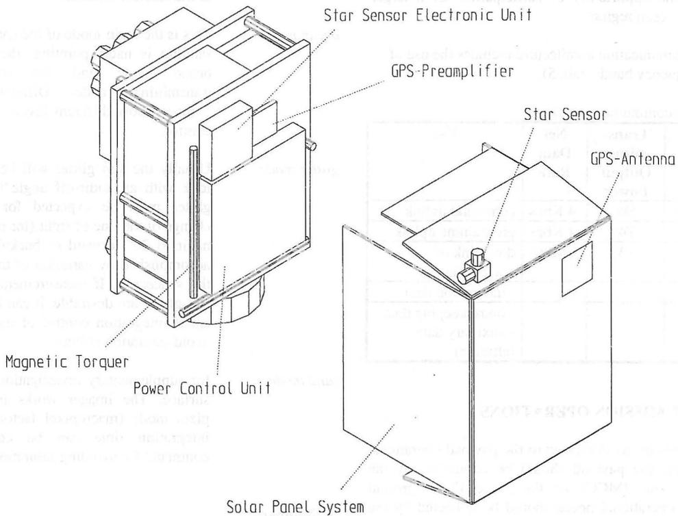
Fig.5: Integration scheme II of the micro satellite
