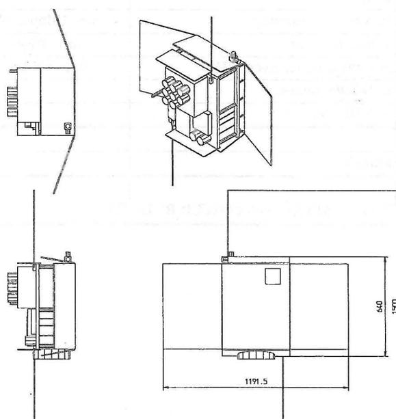
Fig. 3: Flight configuration of the micro satellite
