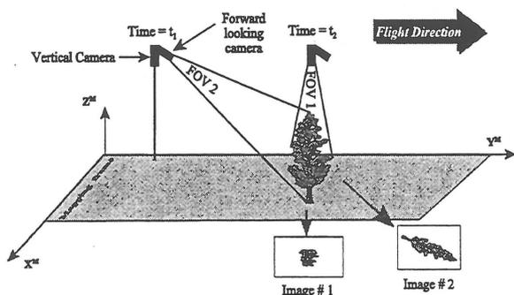
*Figure 10. Vertical and Forward Looking Imaging Component*
