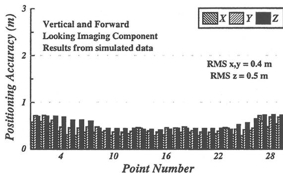
Figure 11. Positioning Accuracy using the vertical and forward-looking imaging component
