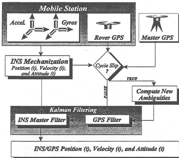
Figure 2. GPS/INS Loosely Coupled Integration Scheme implemented in The KINGSPAD Software of The University of Calgary
