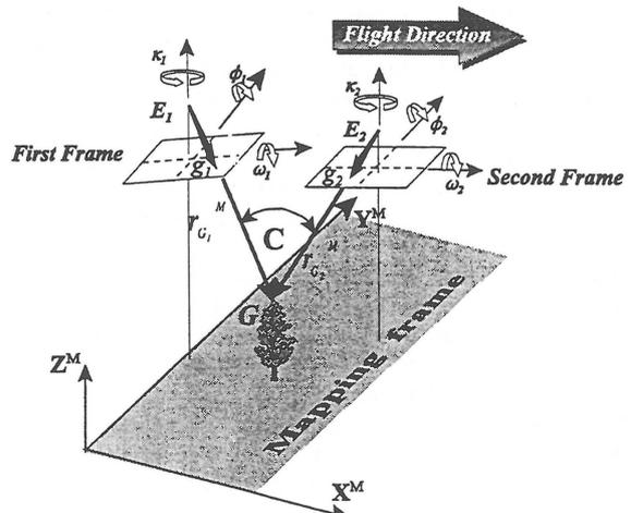
Figure 8. Angle of Convergence between two overlapped frames and an arbitrary ground object (separation between the two frames is exaggerated for purpose of illustration)
