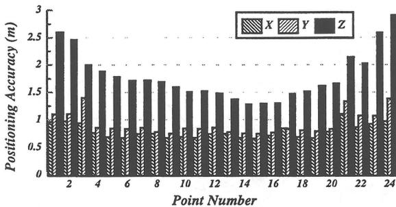
Figure 6. The Multi-Sensor System Overall Accuracy derived from comparing the coordinates of known 24 GCPs with those obtained from direct georeferencing by GPS/INS
