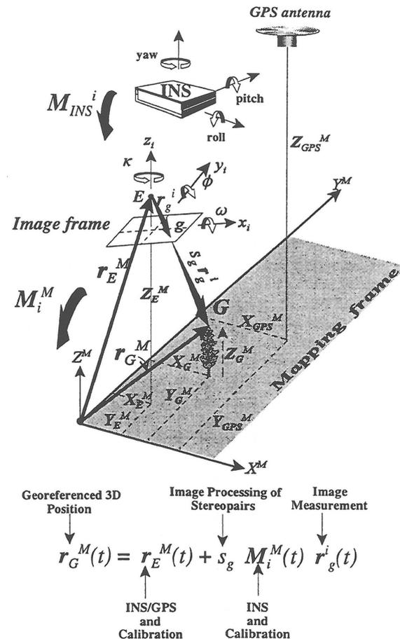
**Figure 1. Georeferencing of a Digital Image by GPS/INS**
