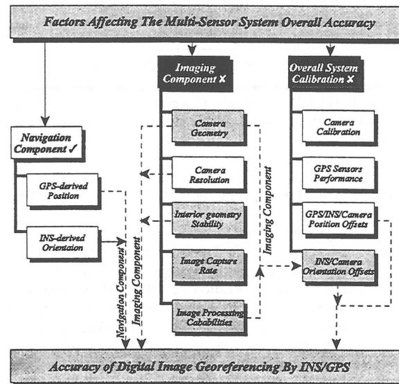
Figure 7. Factors Affecting the Multi-sensor System Overall Accuracy
