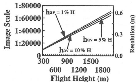
Figure 3. The DCS 420 Digital Camera Average Image Scale and Physical Resolution for Different Flying Heights and Mean Terrain Elevations
