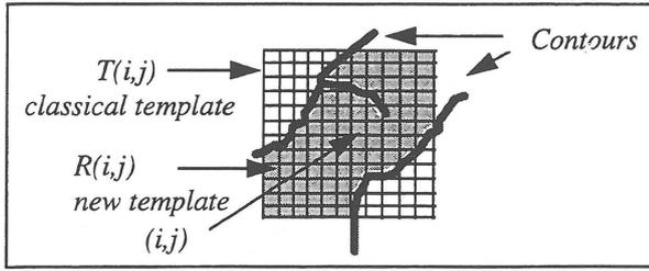
Figure 2-2: Contour adaptive window shape  $S(i,j)$  made from classical rectangular template window  $T(i,j)$ . This pattern is built in the slave image.
