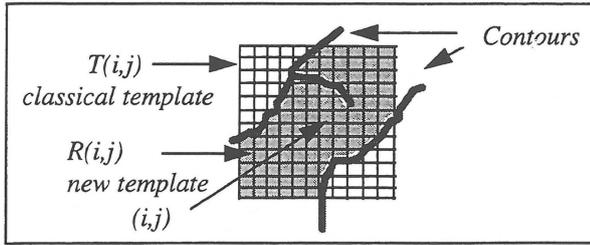
Figure 2-2: Contour adaptive window shape  $S(i,j)$  made from classical rectangular template window  $T(i,j)$ . This pattern is built in the slave image.
