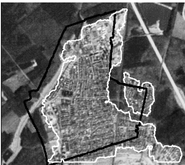
Figure 15: Detail of Fig. 11 with detected built-up areas (white) and GIS data (black).
