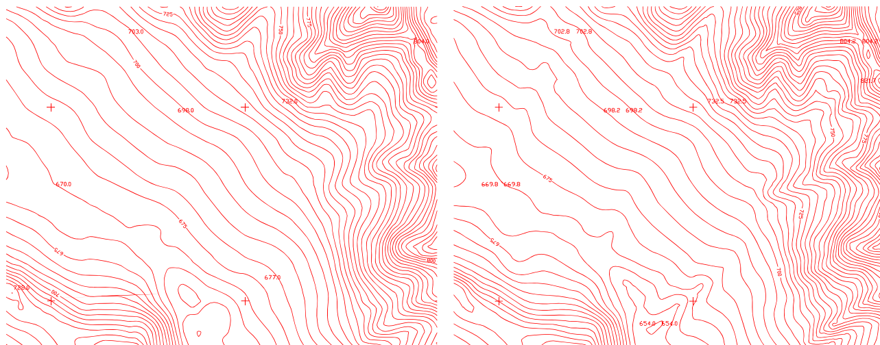
Fig. 3-8: Left: derived contourlines from DTM without additional input. Right: DTM with additional input
