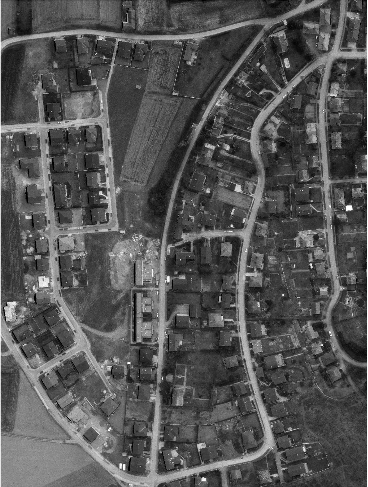
Figure 7: Merged and mosaicked true orthophoto of a suburban area
