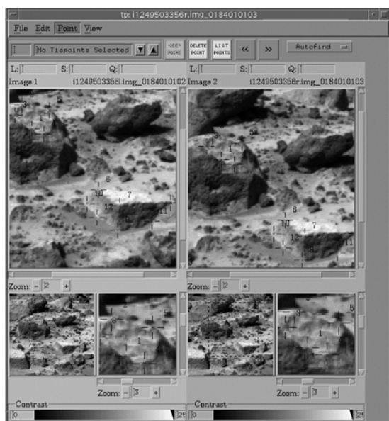
Fig. 4: Pathfinder stereo images in the view of the IP tool, designed for manual collection of tiepoints. CCD chip due to the various mirrors in the two optical paths.
