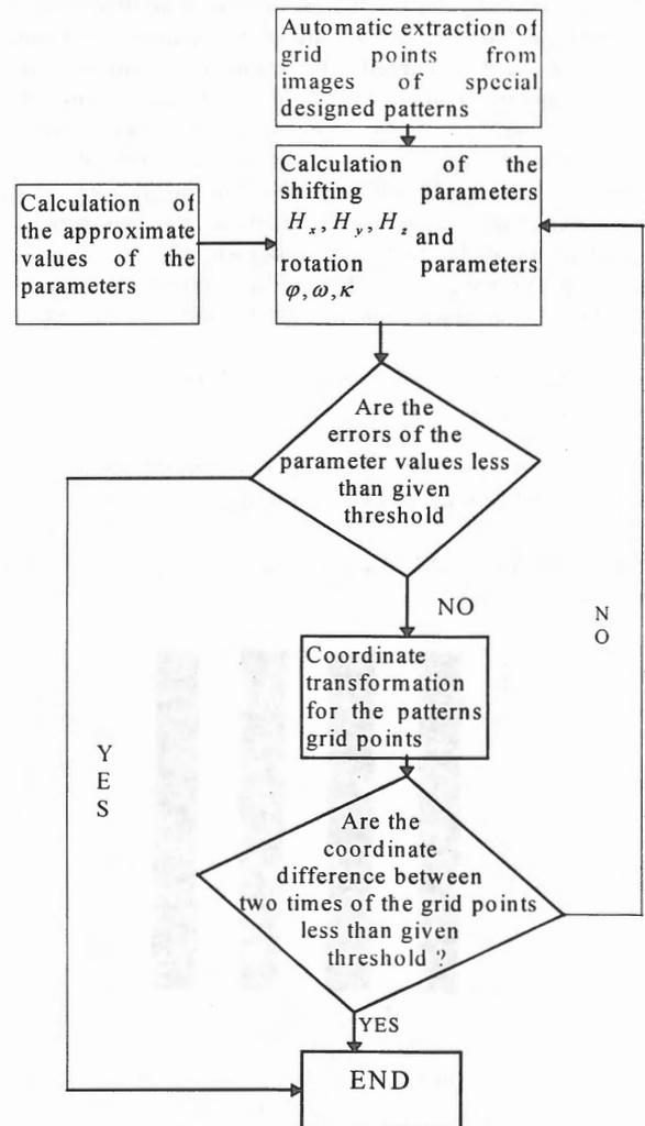
Fig.7 Block diagram of the resolving procedure
