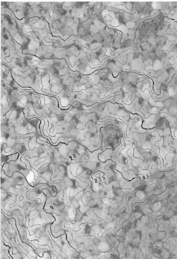
Figure 3: Contoured stereo-model at Display/Edit stage of VirtuZo system processing, during measurement of concrete surface.
