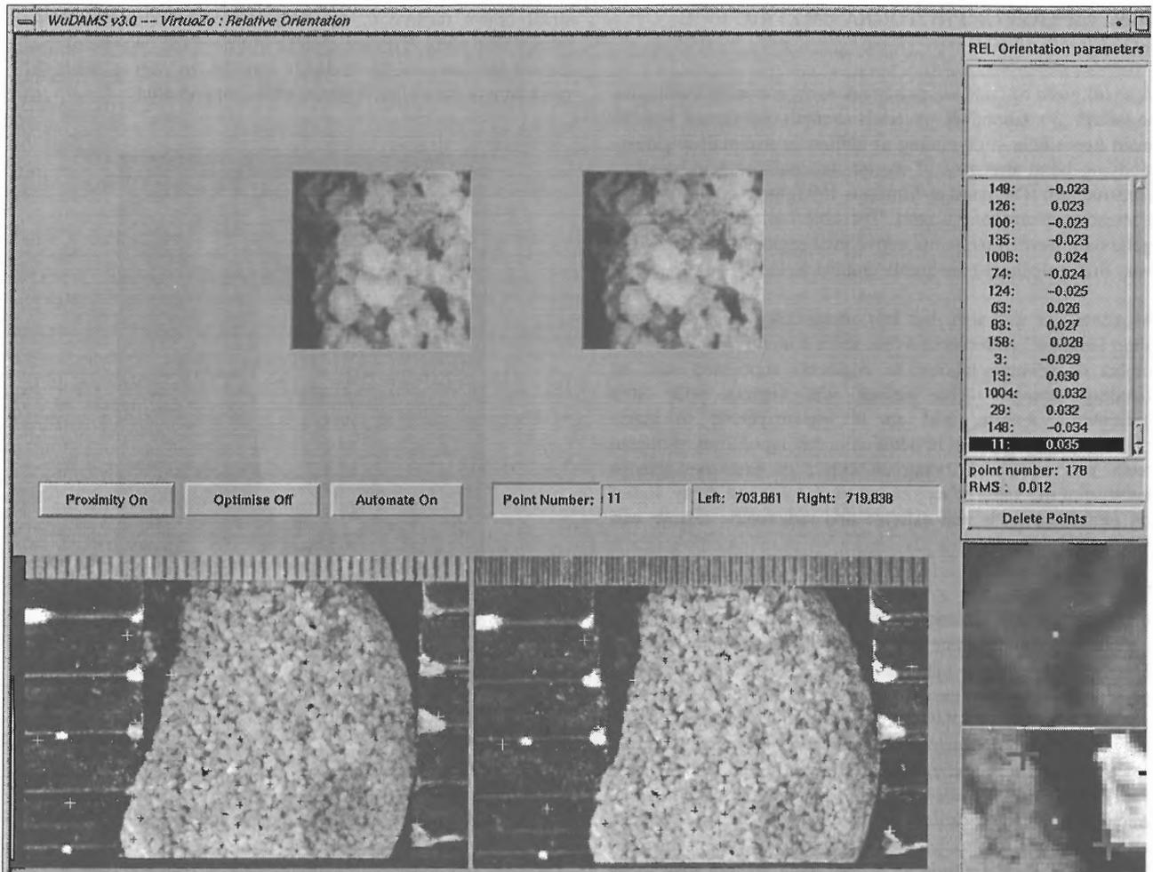
Figure 2: Screen display during relative orientation procedure with the VirtuozO system. The scanned images the concrete break surface are shown, along with close-up views of windows surrounding a point being matched automatically. (The frames may be viewed stereoscopically under good conditions).
