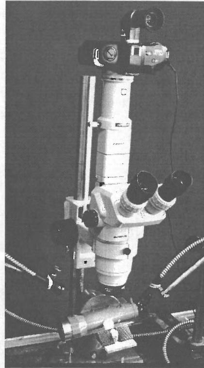
Figure 1: Olympus SZ6045TR microscope, with film camera in position.
