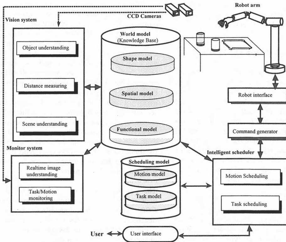
Fig.4 Overall image of knowledge-based autonomous robot system
