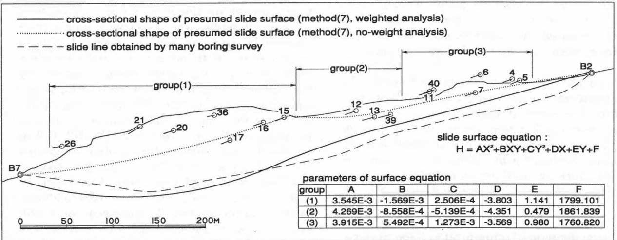
**Fig.11 Cross-section of 3D Slide Surface Obtained by Combination of Many Surfaces (Method 7)**
