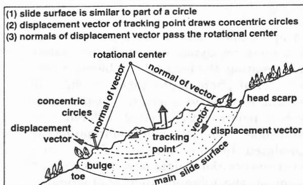
Fig.1 Rotational Slide with Circle [1] (Method 1)
