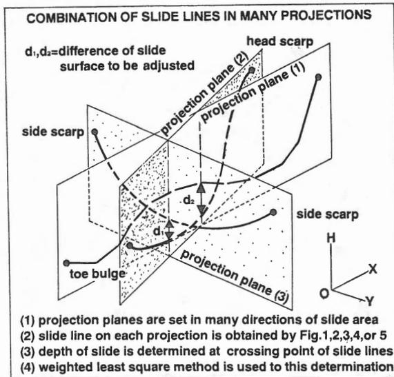
**Fig.8 Combination of Slide Lines (Method 8)**
