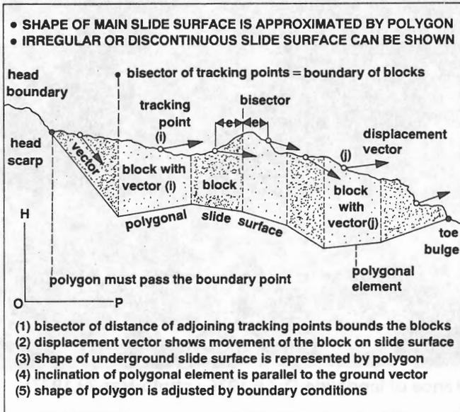
**Fig.4 Slide Surface by Polygonal Shape (Method 4)**
