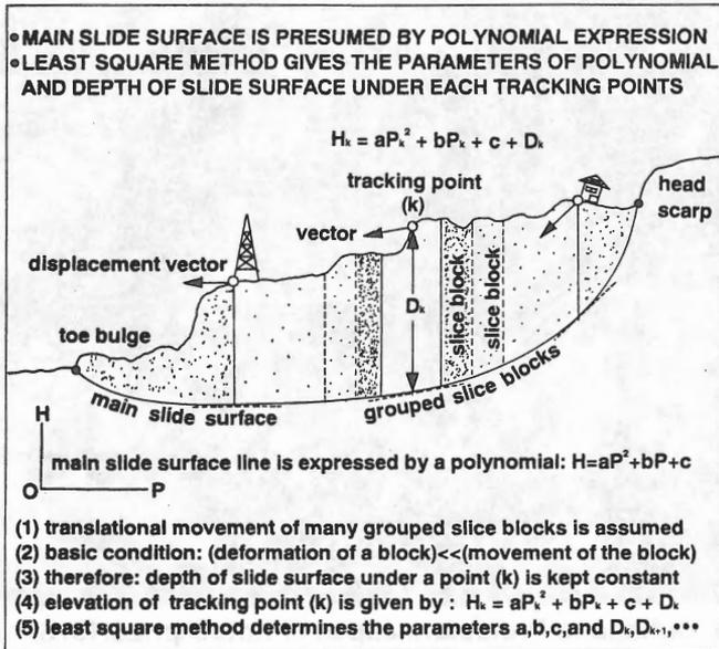
**Fig.3 Slide Surface by Polynomial Curve (Method 3)**
