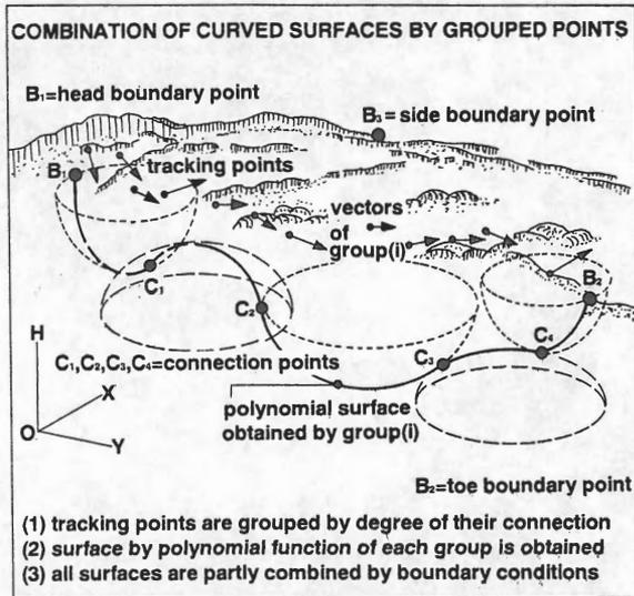
**Fig.7 Combination of Surfaces (Method 7)**
