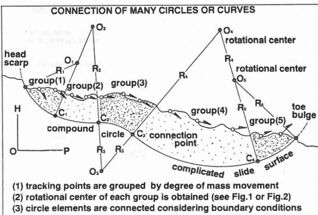
**Fig.5 Connection of Circles or Curves (Method 5)**
