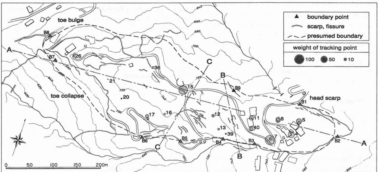
**Fig.12 Weight of Tracking Points Used in Analysis / Presumption of Landslide Boundary Line**
