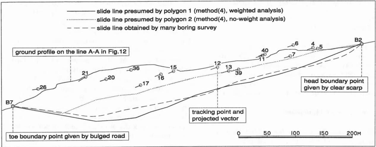
**Fig.10 Shape of Underground Slide Surface Analyzed by Polygonal Curve Fitting (Method 4)**
