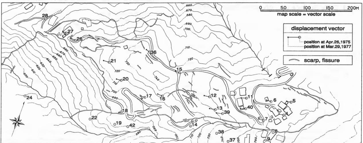
Fig.9 Topographic Map / Displacement Vectors of Tracking Points / Ground Fissures and Scarps
