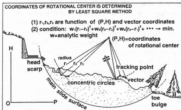
Fig.2 Rotational Slide with Circle [2] (Method 2)
