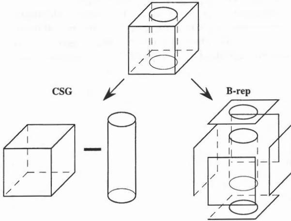
Figure 2: An object modeled with CSG and B-rep
