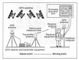
Figure 1. The GPS navigation-type surveying system
