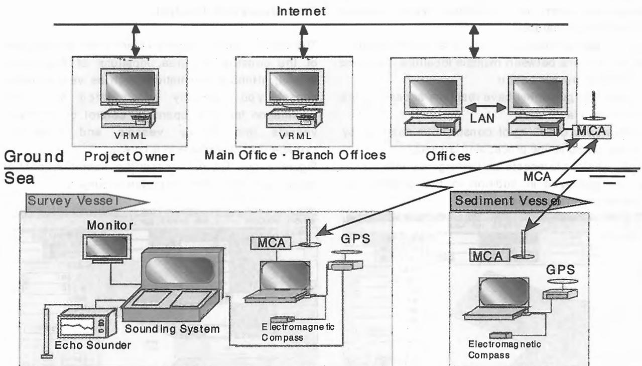
Figure 2 Configuration Diagram of the System
