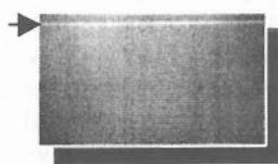
Figure 2: Line Defect
