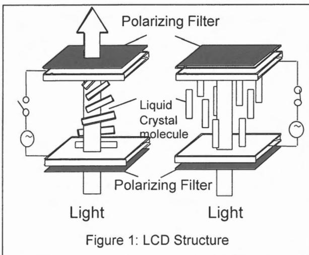
Figure 1: LCD Structure
