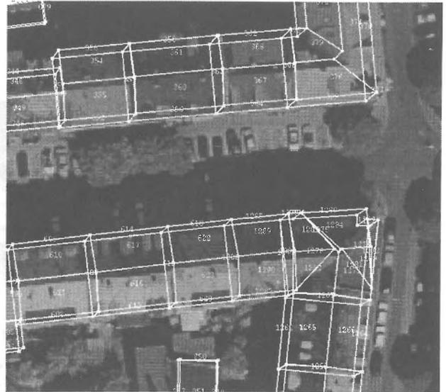
Figure 10: Reconstructed buildings projected into stereo image.
