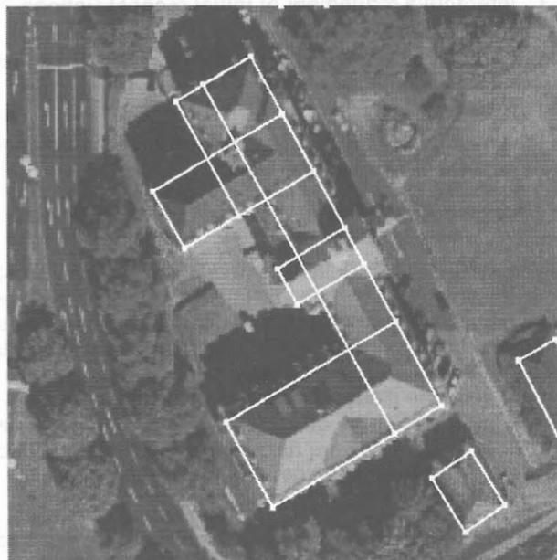
Figure 4: Ground plan decomposed into rectangular parts.
