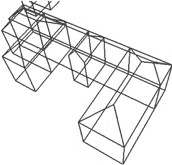
Figure 5: Reconstructed CSG representation.
