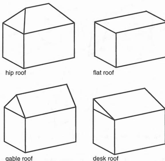
Figure 3: Building primitives used for reconstruction.
