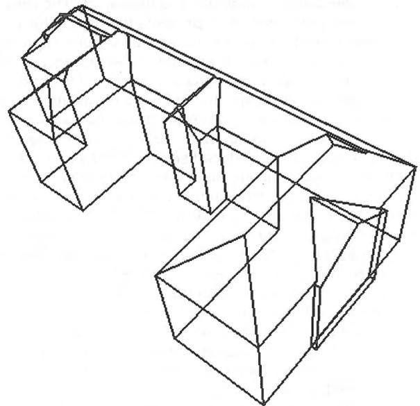
Figure 8: CSG representation of figure 5 transformed to B-Rep (additional bay from interactive refinement).
