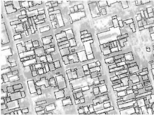
Fig.8 Result of overlapping road polygon with image
