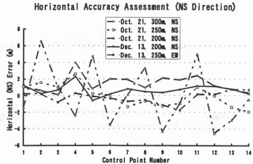
Figure 5. Horizontal accuracy assessment result for ALSS data in the north-south direction.
