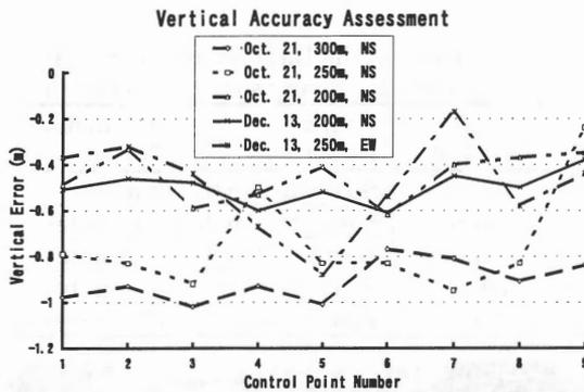
Figure 3. Vertical accuracy assessment result for ALSS data.
