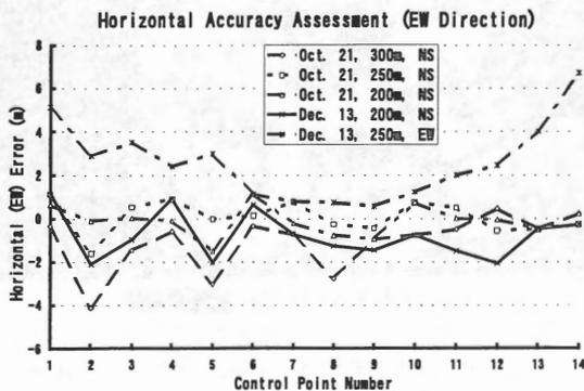
Figure 4. Horizontal accuracy assessment result for ALSS data in the east-west direction.
