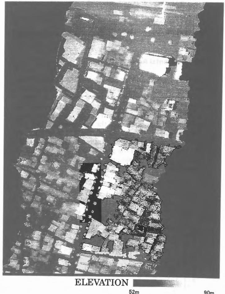
Figure 2. An example of ALSS data of the study area (Acquisition date: October 21, 1996; Flying height: 250m). The arrows indicate the direction of EW flights.
