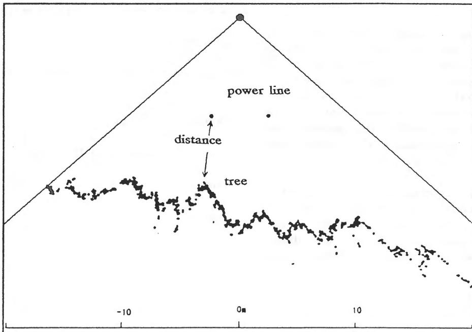
Fig-3. Cross section
