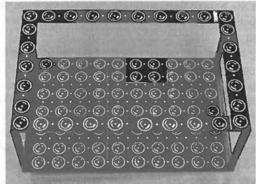
Fig. 6: 3-D calibration frame with coded targets
