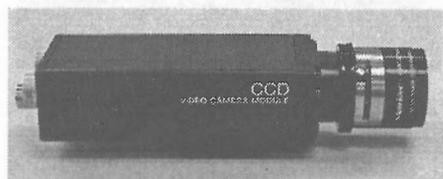
Fig. 2: CCD camera with 35 mm lens
