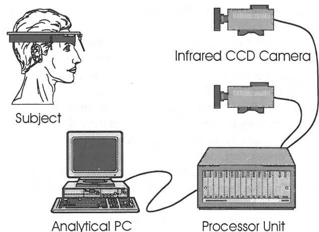
Fig.1 Motion Capture System
