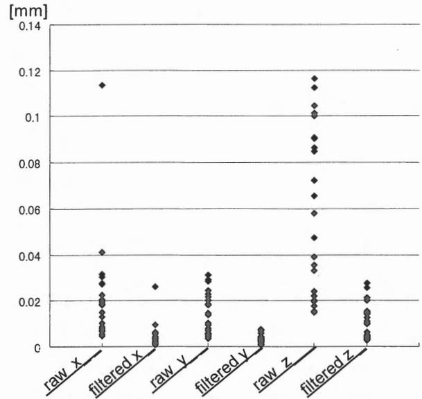
**Fig.3** Difference of Standard Deviation of the Twenty-four Targets on the Grid Before and After Filtering
