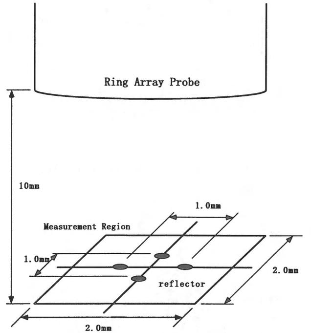
Figure 7: Arrangement of Ring Array Probe and Reflectors
