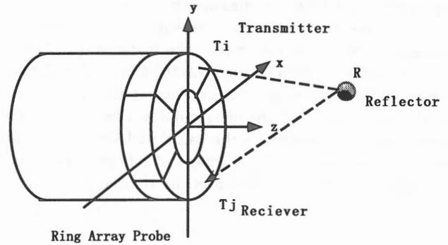
Figure 5: Transmission and Reception of Ultrasound
