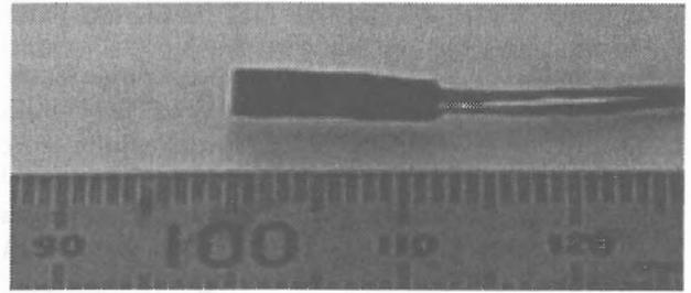
Figure 4: Photo of Ring Array Probe
