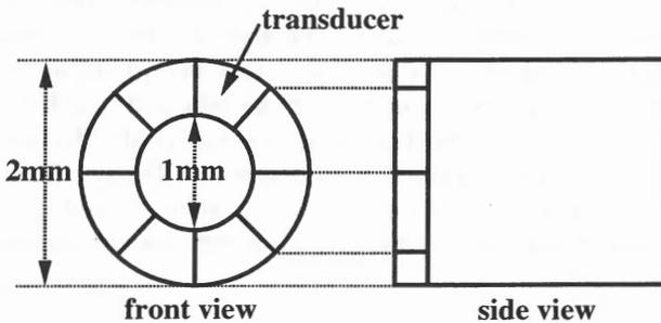
Figure 3: Structure of Ring Array Probe
