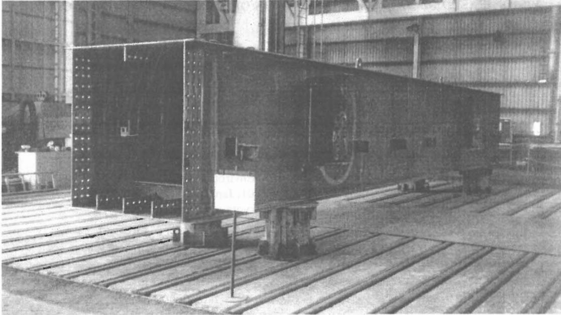
Figure 1: Sample hollow box section or 'bridge block'.
