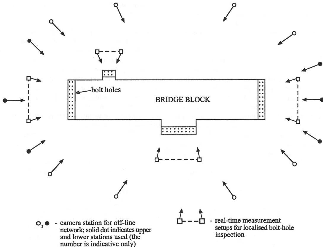
Figure 2: Indicative imaging geometry for a combined off-line and real-time VM inspection.
