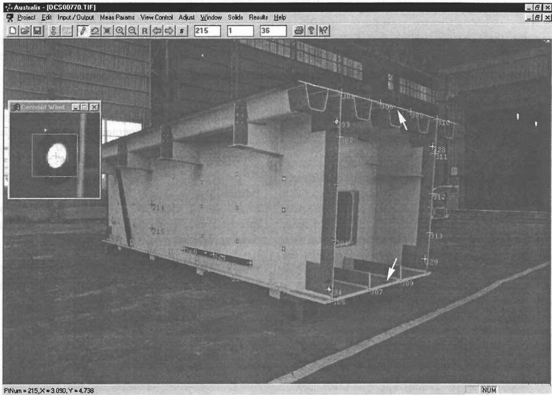
Figure 3: Bridge block used in test inspection, shown in the AUSTRALIS image measurement environment.
