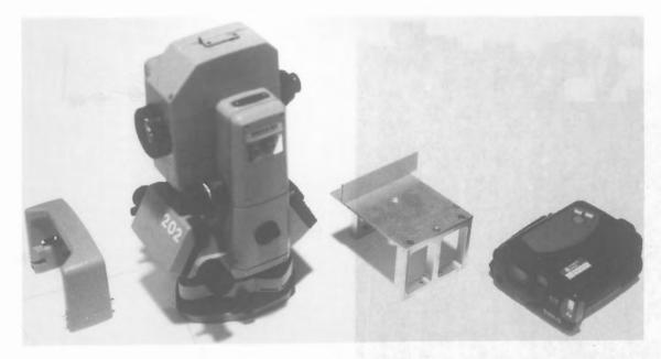
Figure 1 - Total Station, Adapter and Digital Camera
