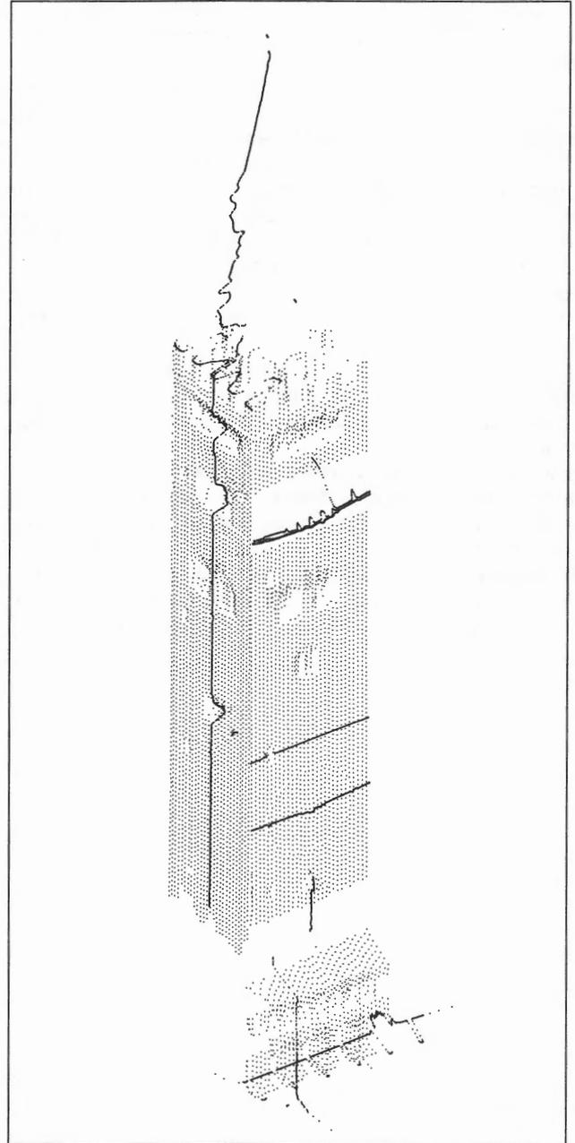
*Topographic detail points surveyed by Autoscanning Laser System MDL*
