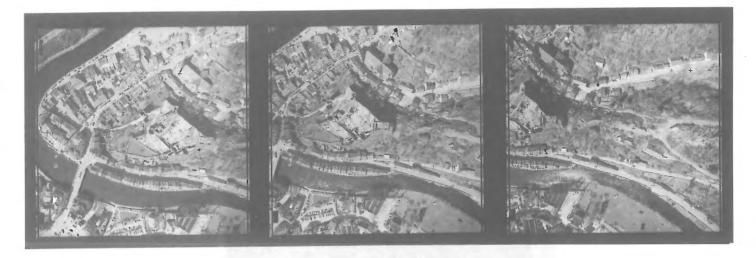
Castel of La Roche en Ardennes : The time lapse calculated in order to obtain 55 to 60 °/° overlap (Rollei Metric 6008).
