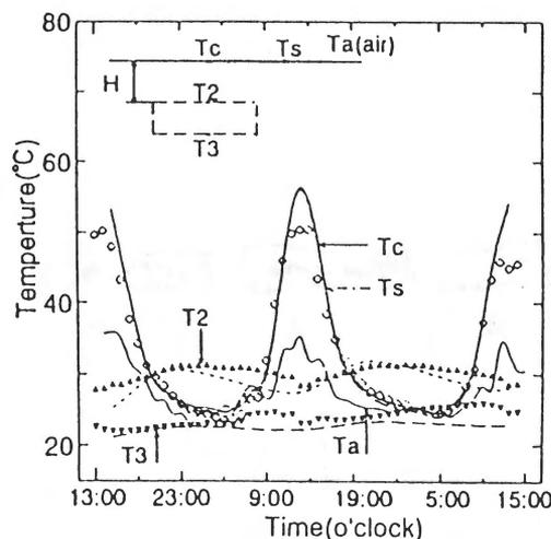
Figure 2 shows the transient experimental and numerical temperatures of the buried plate of H=15 cm in deep. The two temperatures are nearly similar to each other. The numerical calculation represents that the two-dimensional calculated result is possible to simulate the experimental result.
