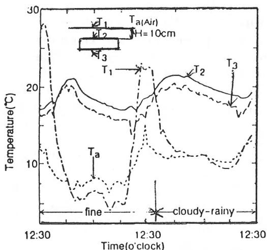
Figure 2 Experimental and numerical temperatures of the buried plate (depth  $H=15 \text{ cm}$ )
