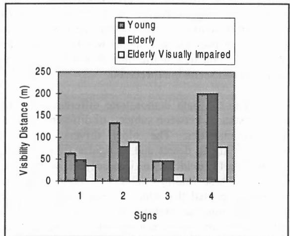
**Figure 4.** Visibility distances measured for a series of traffic signs under nighttime conditions.
