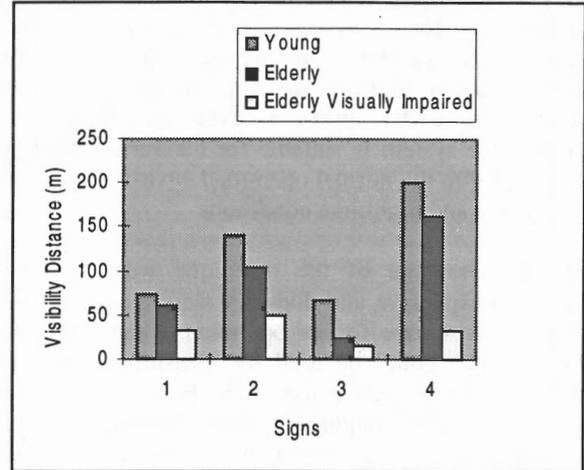
**Figure 3.** Visibility distances measured for a series of traffic signs under daytime conditions.
