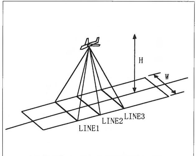
Figure 1 Aircraft loading type TLS
