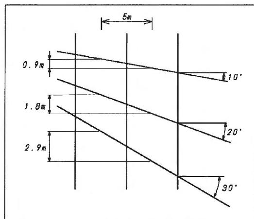
Figure 7 The deviation of the position by the angle of the road and the line
