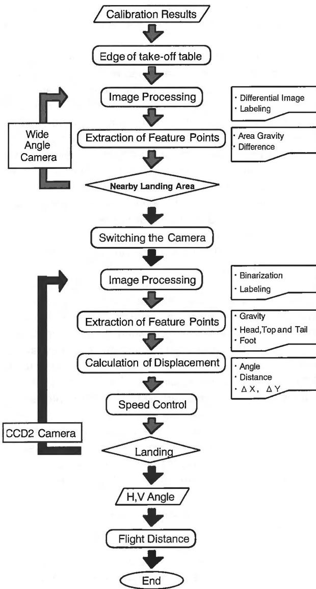
**Figure6 Image processing procedures**
