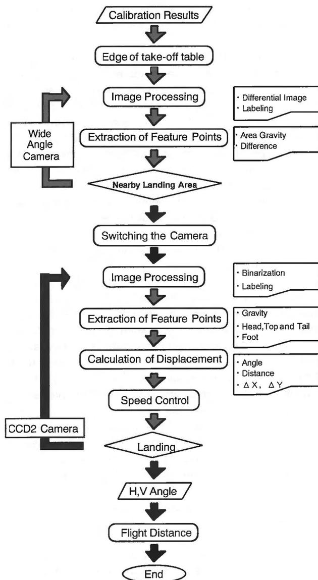
Figure6 Image processing procedures
