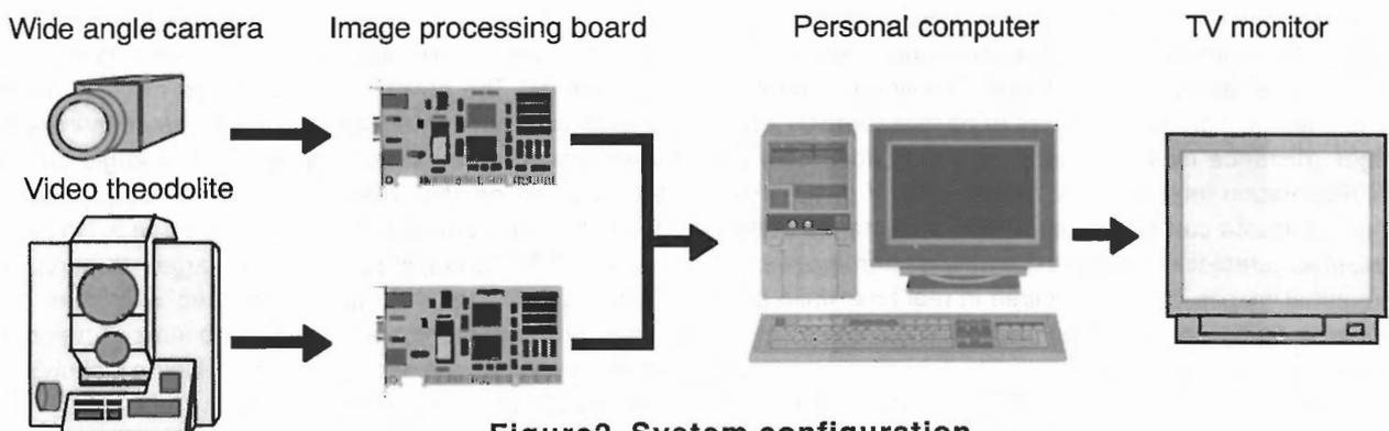
Figure2 System configuration
