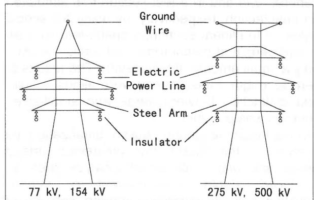
Figure 3. transmission lines tower
