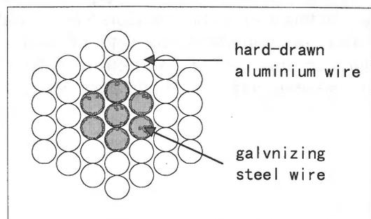
Figure 4. cross section of steel feeling aluminium wire
