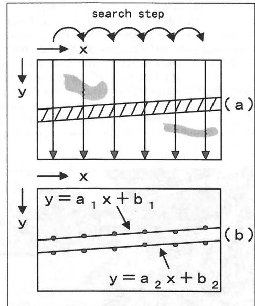
Figure 8. ground wire detection method
