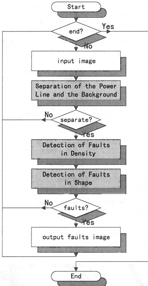
Figure 7. detection of faults flow
