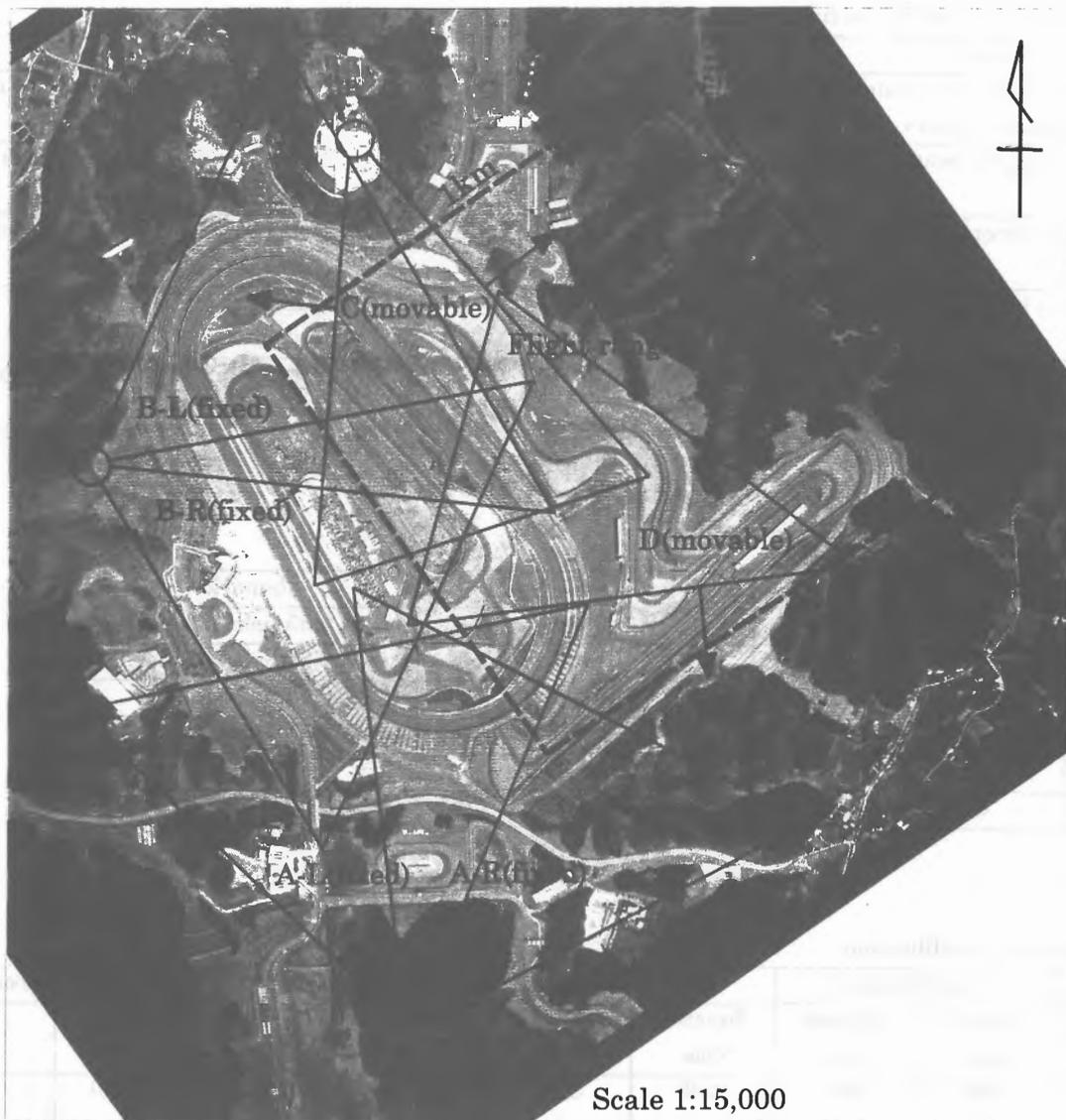
Figure 1 : Flight range of airplane and location of video cameras
