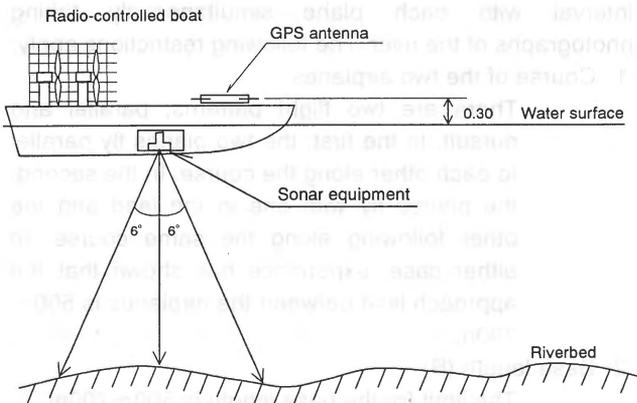
Fig.3 Measurement method using radio-controlled boat
