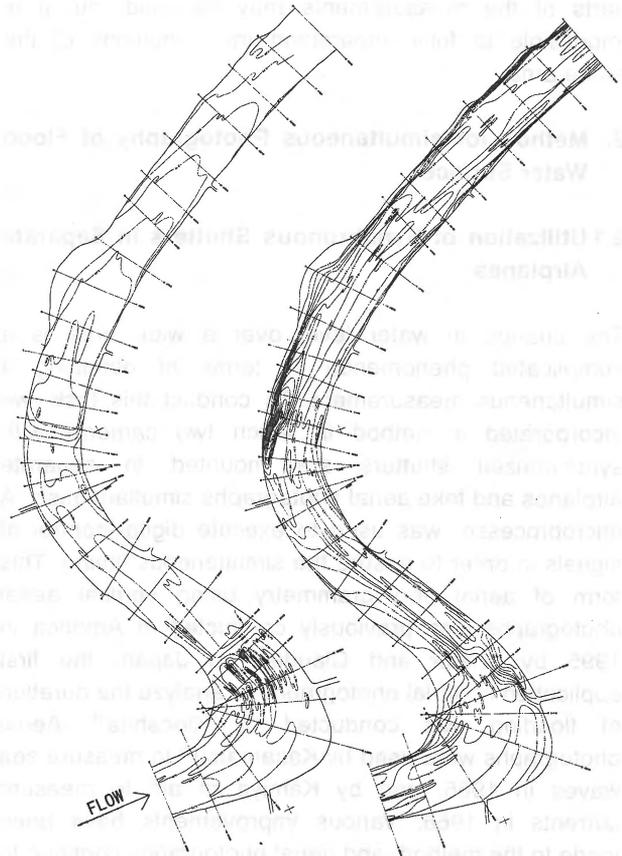
Fig.4 The contour line map of flood flow surface
