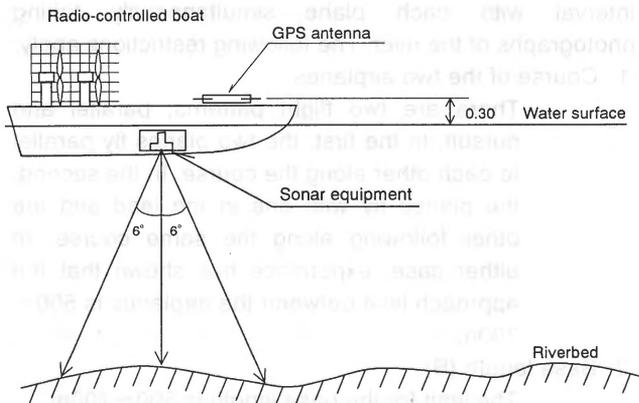
Fig.3 Measurement method using radio-controlled boat
