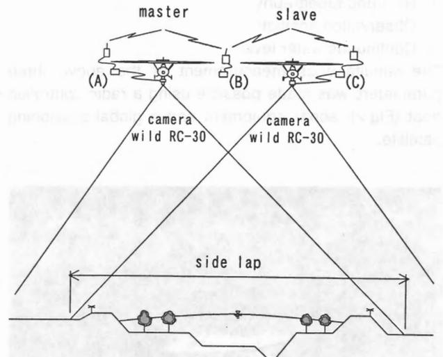
Fig.9 Method for simultaneous photography of flood water surface
