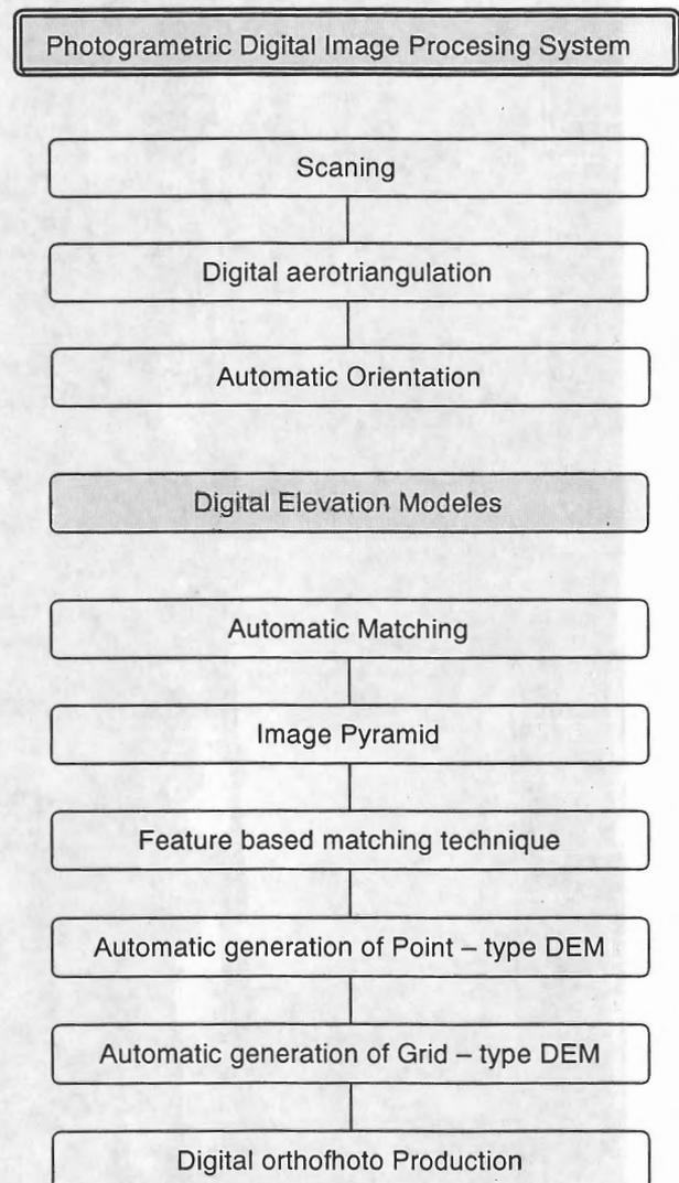
Fig.10 Flow chart of photogrammetric digital image processing system
