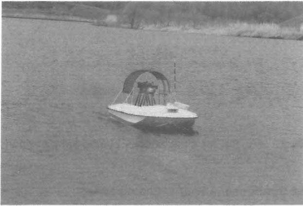
Fig.2 Radio-controlled observation boat
