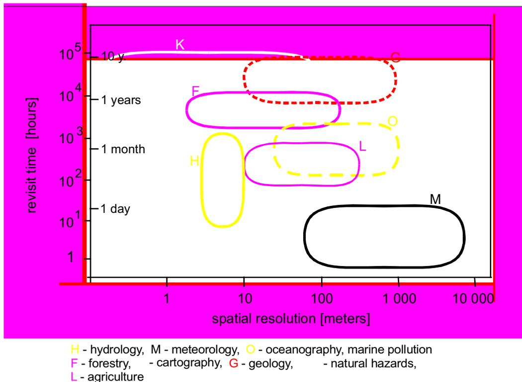
Figure 2: Spatial resolution and revisit time for different remote sensing tasks
