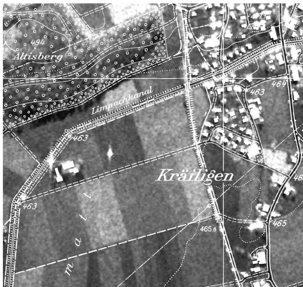
Figure 2: Terrain-geocoded SAR scene of an area near Solothurn with superimposed topographic map (scale 1 : 10,000)
