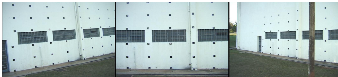
Figure 3 - Convergent calibration method.
