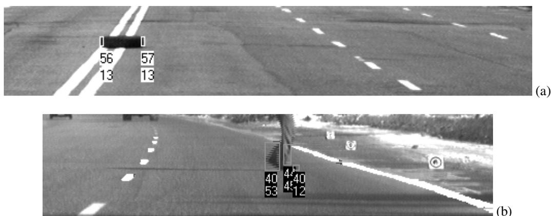
Figure 7. Examples of detection. (a) A car tire. (b) A pedestrian.
