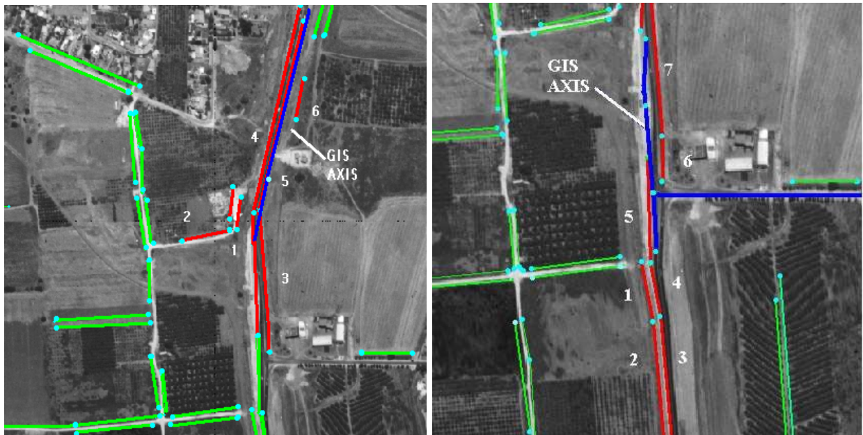
Figure 4: GIS data (blue) and hypothesized road features (red and green) overlaid on an orthophoto. Marked GIS segment is matched with red image segments.
