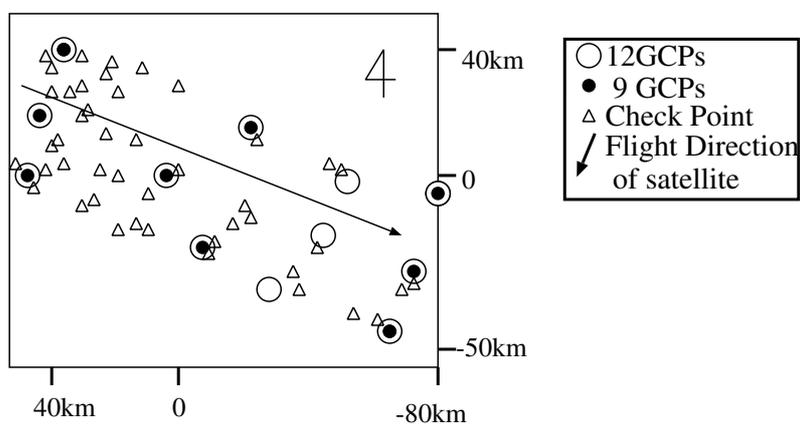
Figure 4: Disposition of GCPs and Check Points for MOMS-2P images
