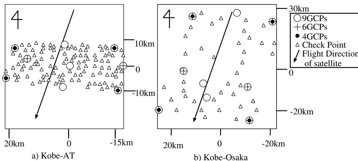
Figure 3: Disposition of GCPs and Check Points for Kobe-AT and Kobe-Osaka
