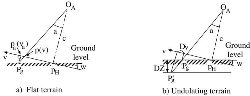
Figure 1: Image transformation from central perspective to affine projection
