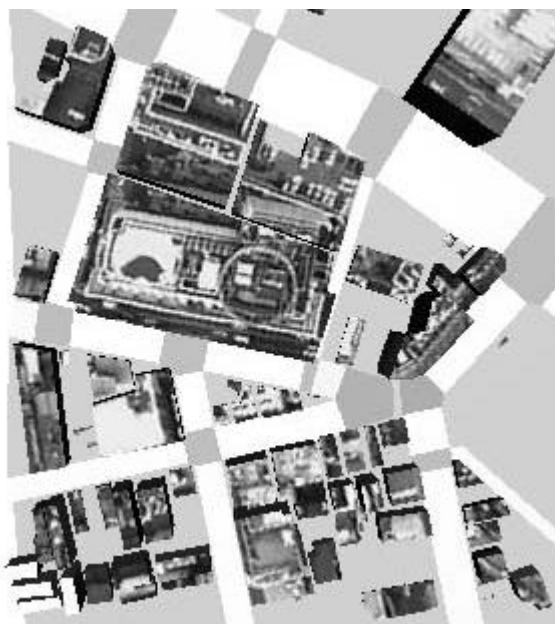
Figure 10. 3D digital city model projected texture acquired from video images
