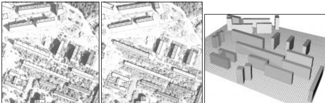
Figure 8. Example of building reconstruction: left image of stereo-pair with extracted roof edges (at the left), right image of stereo-pair with extracted roof edges (at the center) and reconstructed 3d model (at the right)
