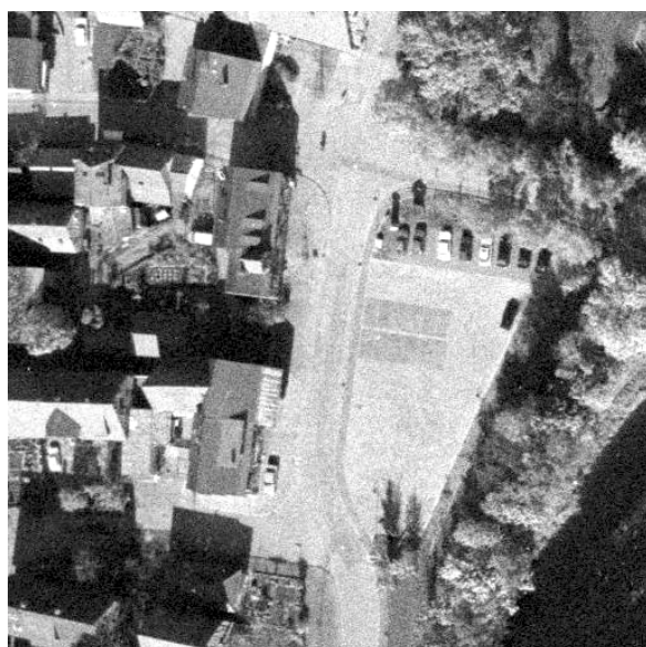
Figure 4: RMK image (scanned at 15 µm resolution, flying height 2000 m, GSD 20 cm)
